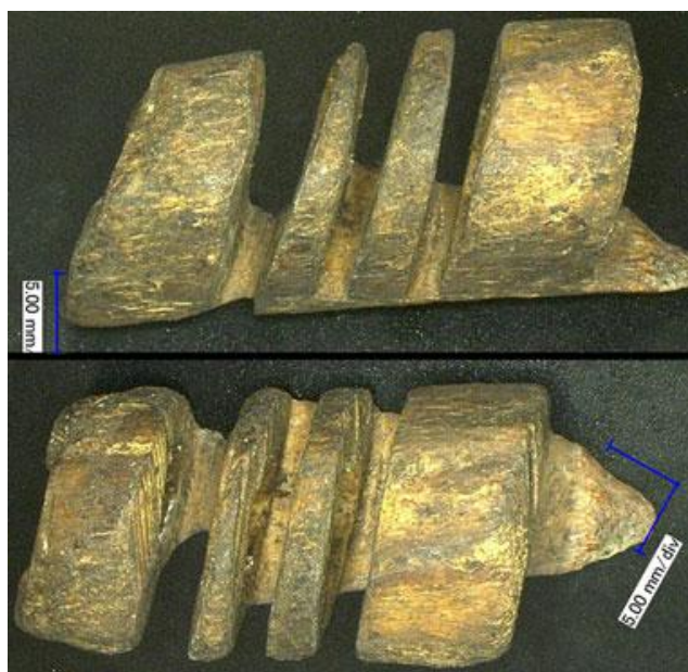
Figure III-25. Two views of numerous identical false starts, which are too uniform for a hand saw.
